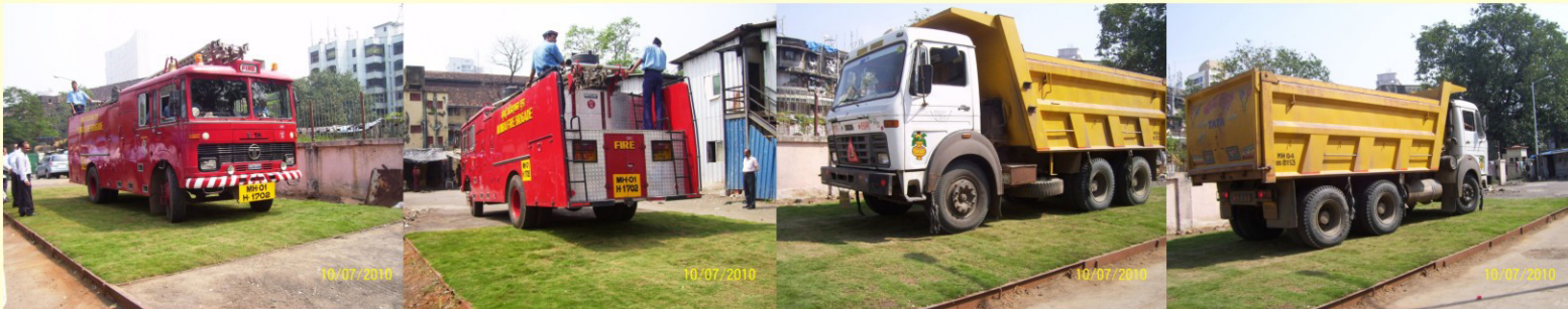
Load test done by Mumbai Fire Brigade with the load of 16 Ton fire tender at K. Raheja site in Mumbai.
